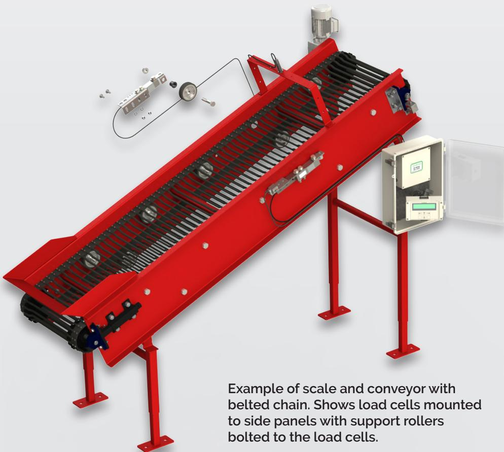
Example of scale and conveyor with belted chain. Shows load cells mounted to side panels with support rollers bolted to the load cells.
